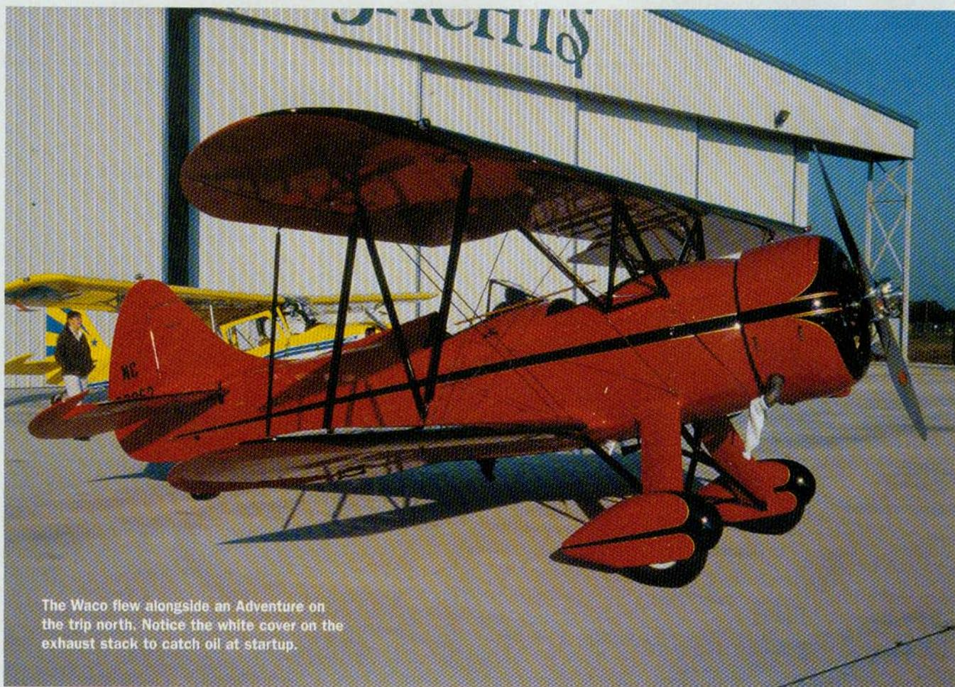
The Waco flew alongside an Adventure on the trip north. Notice the white cover on the exhaust stack to catch oil at startup.
