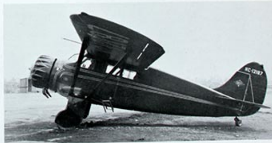
R-3 featured retractable landing gear, 240-hp Lycoming. Engineer/test pilot R. W. Ayer nearly forgot to lower prototype 449M's gear for first landing. NC12187, below, had special cowl with rocker-box blisters. Only five R-3's were built.
