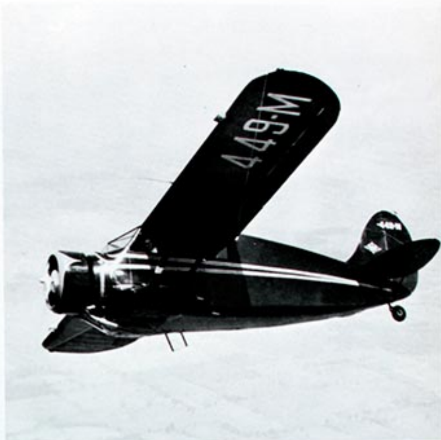
R-3 featured retractable landing gear, 240-hp Lycoming. Engineer/test pilot R. W. Ayer nearly forgot to lower prototype 449M's gear for first landing. NC12187, below, had special cowl with rocker-box blisters. Only five R-3's were built.
