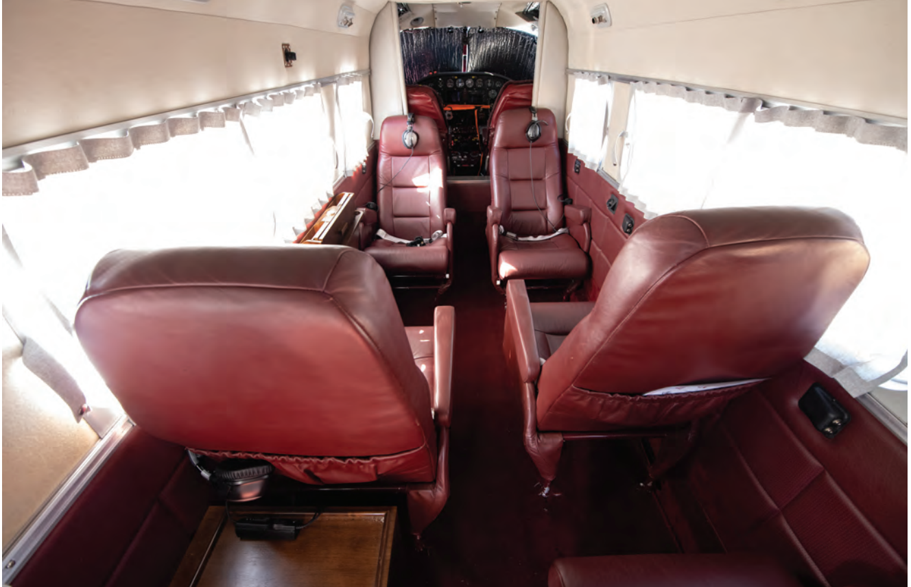
The interior was stripped to the fuselage skins and brought back to the form the President of Mexico enjoyed.
